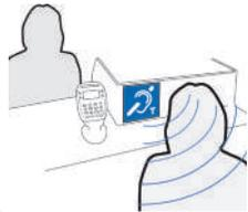
The hearing loop aerial is located within the signage, which is fixed to a counter, desk or glass surface to enable your customers to easily identify the loop and get maximum benefit from it. The unit can be fitted into many positions due to its low profile structure.
