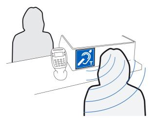
Hearing loop systems overcome this problem. Speech is picked up through a microphone, converted to magnetic impulses by the driver and transmitted via a loop aerial. This magnetic signal is picked up by the telecoil within hearing aids and converted back to speech. Clever stuff!
