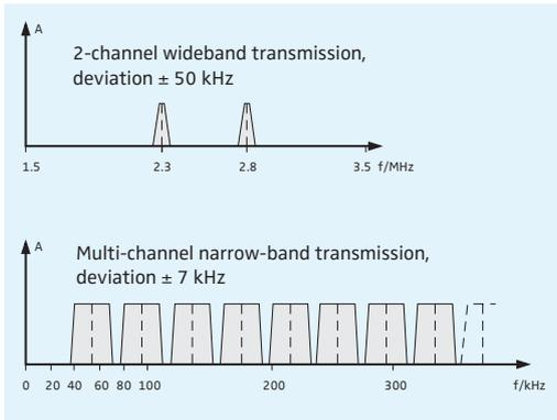
Wideband/narrow-band transmission: modulators and receivers have to use the same principle and operate on matching frequencies!
